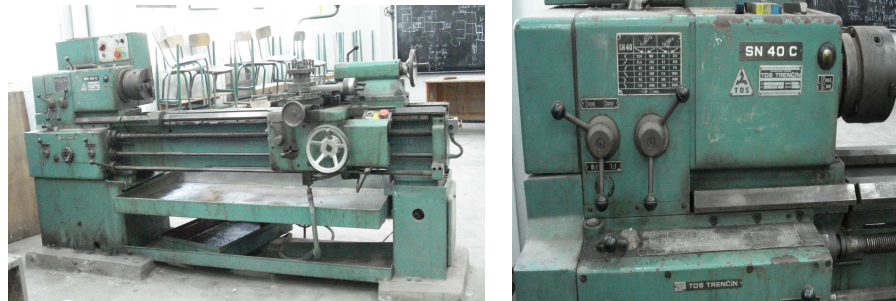
Figure II.2 Tour universel TOSTRENCIN SN40 C
