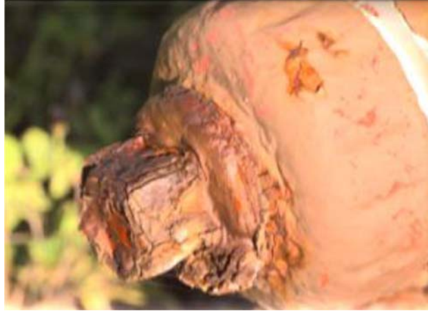
Figure II.5- La corrosion intergranulaire [3]
