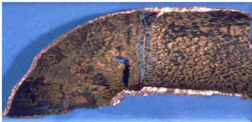
Figure II.4- La corrosion caverneuse [3]
