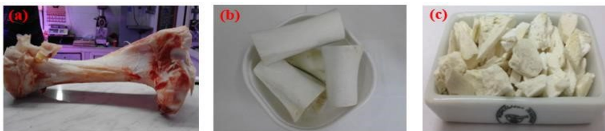
Figure 2. Photographs of bovine femur: (a) Raw state; (b) washed and cleaned; (c) pulverized
