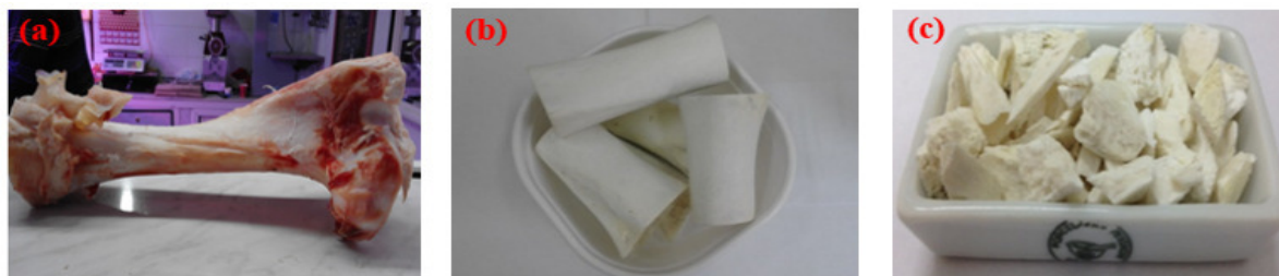
Figure 2. Photographs of bovine femur: (a) Raw state; (b) washed and cleaned; (c) pulverized
